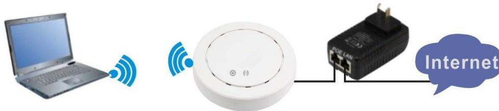
P1 Data transmitted & Powered by PoE Adapter
