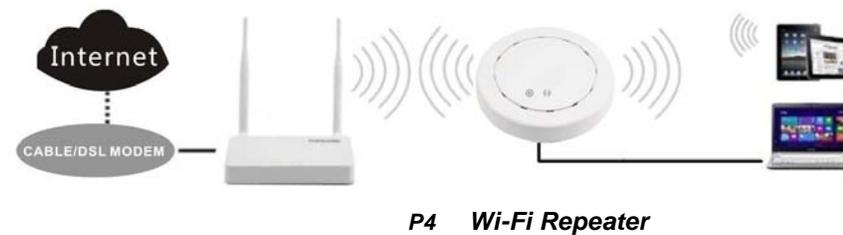
**Wireless AP Mode:** plug and play, suitable for hotel, school, super market and so on. The connection is: the internet cable is connected from router/switch to ceiling AP, then ceiling AP will transmit Wi-Fi signal, PC and end user can access into internet by wired/wireless
