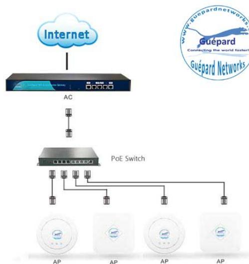
Working diagram as Gateway and AC Controller
