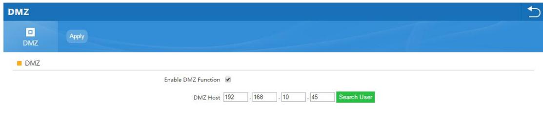
The screenshot shows the DMZ configuration page. At the top, there is a blue header with the word "DMZ" and a back arrow. Below the header, there is a navigation bar with "DMZ" and "Apply" buttons. The main content area has a sub-header "DMZ" and a checkbox for "Enable DMZ Function" which is checked. Below this, there are four input fields for the DMZ Host IP address: "192", "168", "10", and "45". To the right of these fields is a green "Search User" button.
