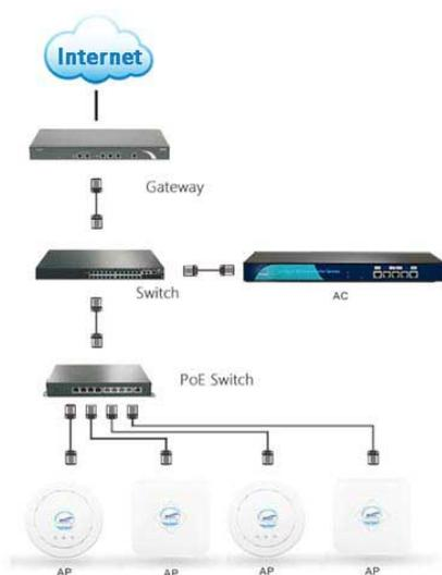
Working diagram as AC Controller
