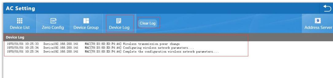
When finish the Address Server, Zero Config and Device Group, can connect wireless AP into this network.
